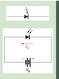
The photodiode allows essentially no reverse current (except for a very small dark current) when there is no incident light.
